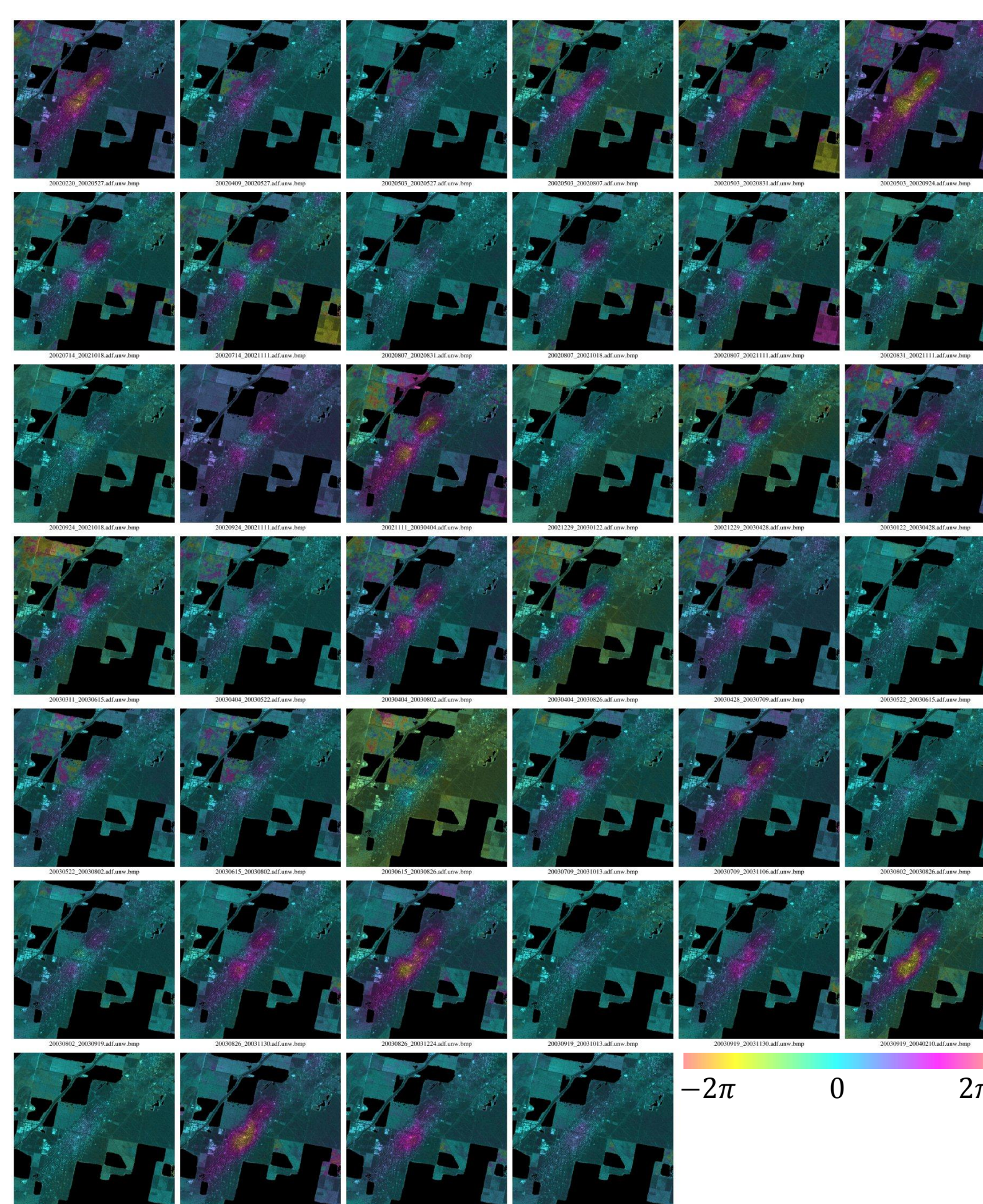
Figure 3. Unwrapped interferograms showing atmosphere and deformation phase
